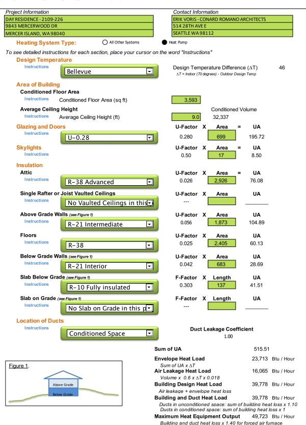
Building and duct heat loss x 1.25 for heat pump
